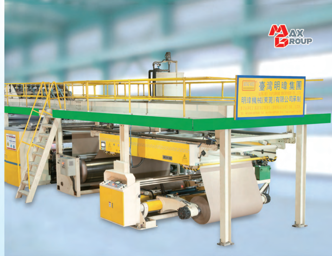
BC-7 Overhead Bridge Conveyor
